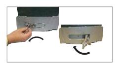
Push the hinged release lever back into the body of the operator and turn the key anti-clockwise a quarter of a turn (90°) to re-lock. Remove the key and replace the dust cover.
