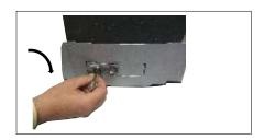
Flip off the grey plastic lock dust cover. Put the key 2 into the lock barrel and turn clockwise a guarter of one turn (90°).
