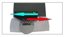
Slowly push the gate in either direction until the operator's drive gears re-engage. 2
