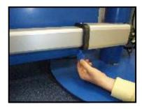
The Mini & Mark Tanks' brass emergency release valve is located on the centre-underside of the operator as indicated by the arrow in the photograph to the left.
