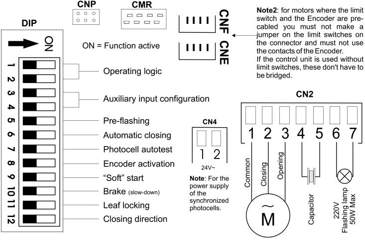
Note3: On the 24V Ph output it is possible to connect a relay for the timed activation of a courtesy light. 67411050 Rev. 01 - 06/2011
