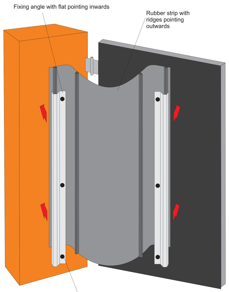
Drill holes anywhere on flat for fixing to gate and pier.
