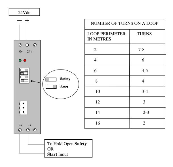
The loop layout drawings below shows a 6 metre perimeter loop cut into tarmac and having 4 turns around the perimeter. Use the chart above to select the correct number of perimeter turns required any given loop.
