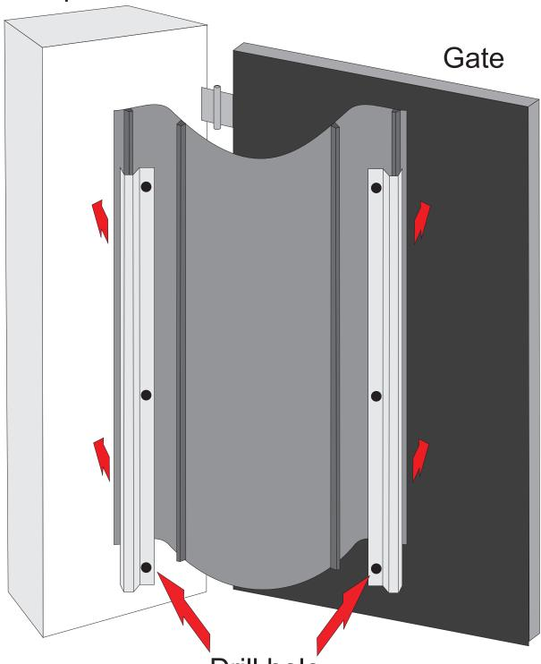
Tech screws will fasten hinge guards to most gates and posts.
