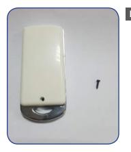
EN Use a screwdriver with a 1.2 mm tip to unscrew the back screw
