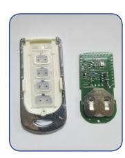
Open case with the help of a coin, to release the cover. Then remove the battery
