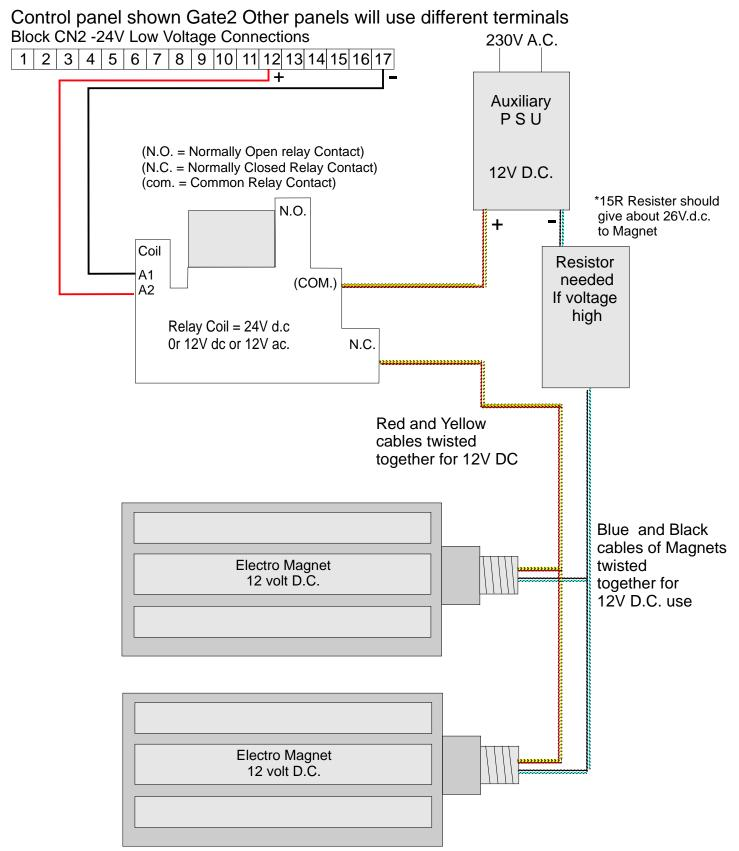
Check magnet wiring diagram for 12v dc cable colours as manufacturers vary
