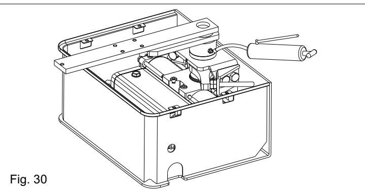
When putting in function the installation it is peremptory to lubricate the box as in Fig. 30 until the grease comes out. (Use grease type DIN 51502 KP 2 N-20 - K2 K-20).
